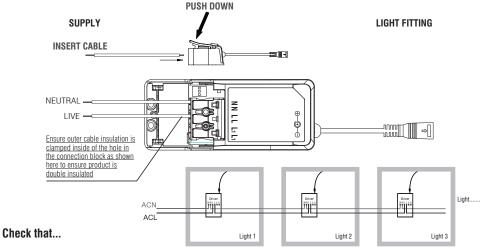
You have to correctly identified the wires.
